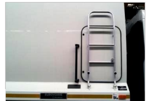
Inspection door with stair and handle
