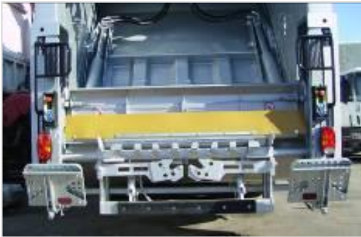
Multi-purpose bin-lifter in down position
