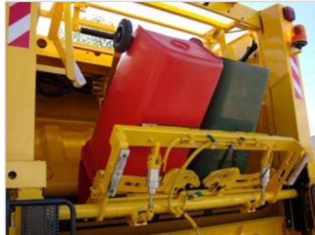
Multi-purpose bin-lifter in lifted position
