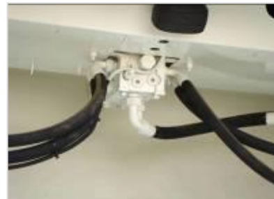
2nd hydraulic block located on the tailgate
