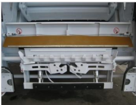
Rail rave in lifted position
