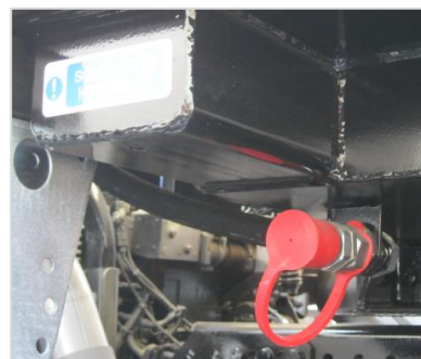
Detail of the push-fit coupling
