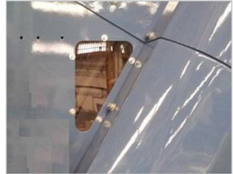
Inspection window on the tailgate
