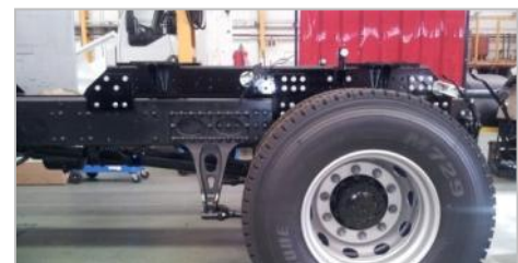
Sub-frame mounted on a chassis
