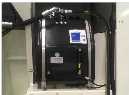
Oil tank at the front of the body
