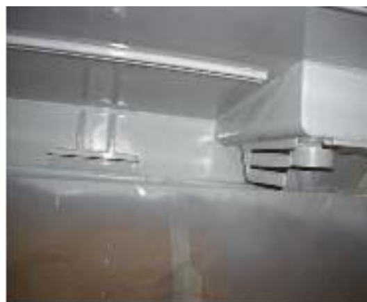
Bottom of the body painted and sealed
