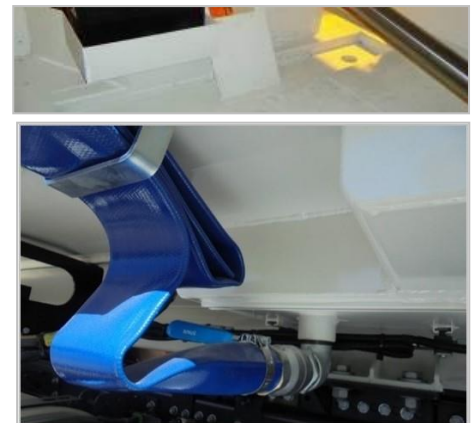
Interior view of the tank and exterior view of the drain hose
