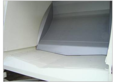
Detail of keel-shaped floor
