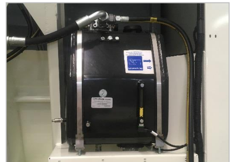
Front view with the oil tank
