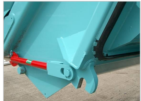
Anchor for locking the tailgate
