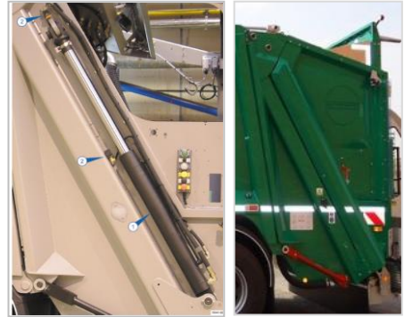
Carriage plate cylinder open and with fairing
