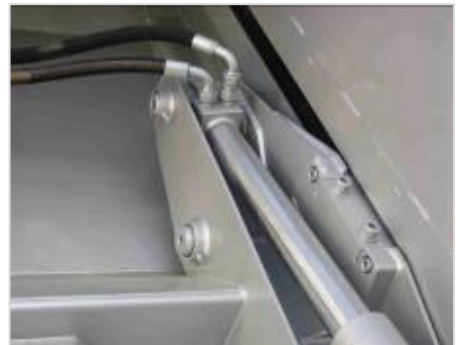
Chrome-plated packer cylinder and rod
