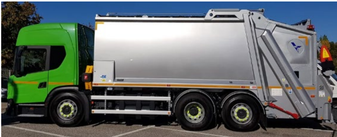
Olympus 20W with Terberg OmniMAX mounted to Scania LPG L280 6x2 E6
