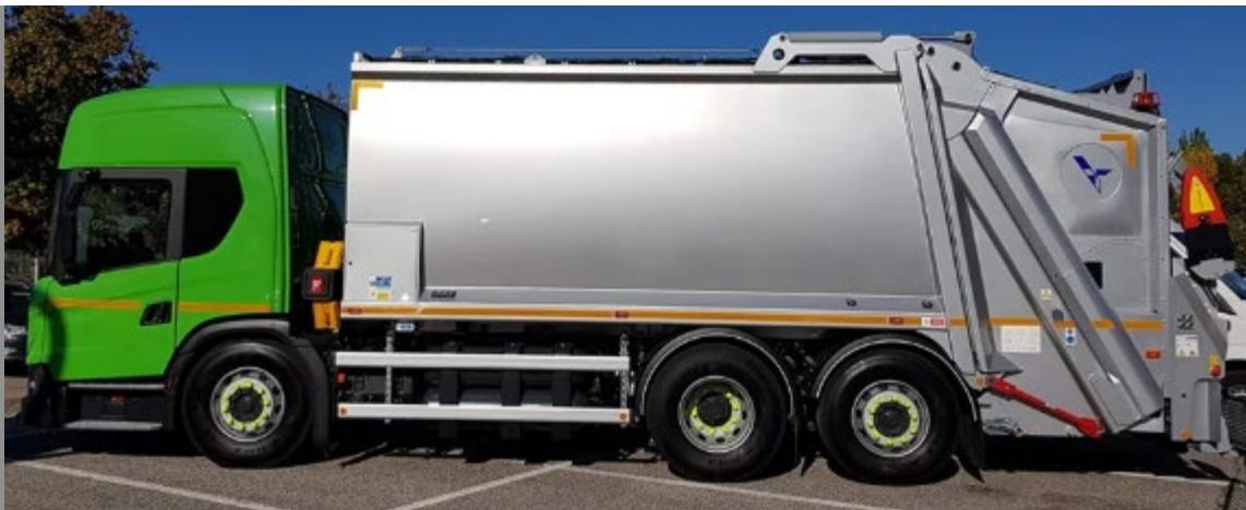
Olympus 20W with Terberg OmniMAX(E) mounted to Scania LPG L280 6x2 E6
