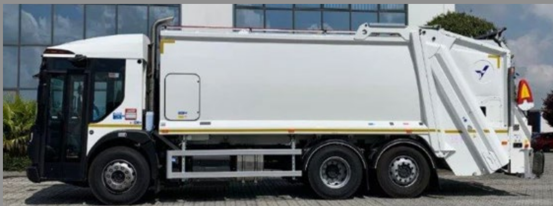
Olympus 21W with Terberg OmniMAX(E) mounted to Renault D-Access 6x2 Rear Steer
