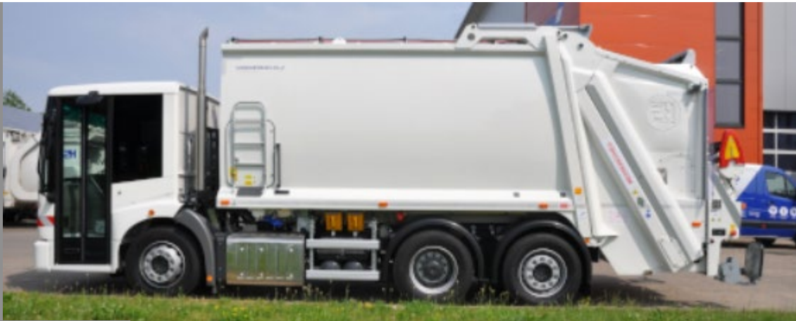
Olympus 20+ with Terberg OmniMAXé mounted to Mercedes Econic 2635L ENA 6x2/4
