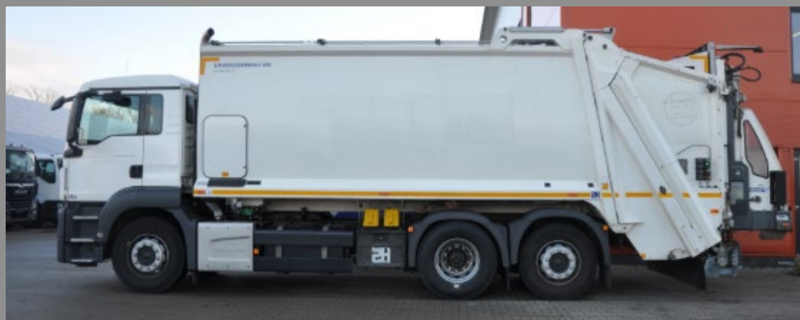
Olympus 25+ with Terberg OmniDE-X mounted to MAN TGS 26.320 6x2-2 BL
