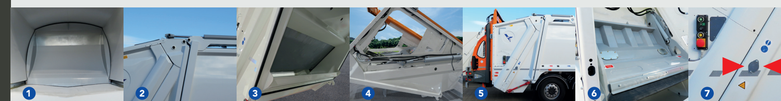
1 Leachate tank at the bottom of the body. Keel shaped floor helps leachate flow to drain sump. 2 Tailgate lift cylinders on the hopper roof 3 Full height tailgate seal 4 External cylinders 5 Minimum overhang 6 High absorption capacity press 7 2 grease points
