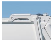
4 Lift cylinders in the hopper roof.
